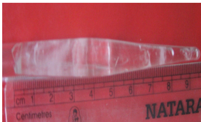
Fig. 1. Photograph of unidirectional grown single crystal.
